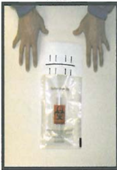
Figure 1: shows the bag laying flat on a counter with the tape side up and the tape end towards the person closing the bag.
