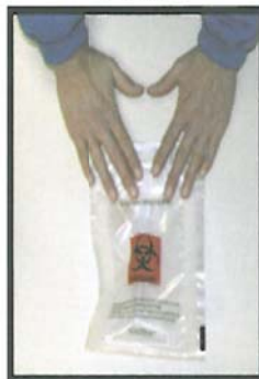
Figure 5: shows the middle finger of both hands being used to press the adhesive together. Start at the center of the fold and work outward. Please be sure to firmly press the entire adhesive area, especially the folded edge and corners.
